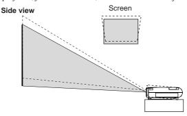
(There is approximately 5 degrees of up and down adjustment for the front of the projector.)
